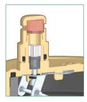
The operating principle of the hydroscopic cap is based on the properties of the cellulose fibre discs forming part of the retaining cartridge.
