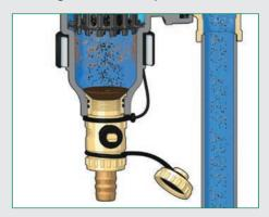
The collected debris can be discharge from the DISCALDIRTMAG whilst the system is in operation by removing the magnet, opening the blow down valve and flushing through the debris.
