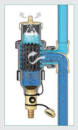
Dirt separators operate by a combination of physical principles. The internal element is constructed to form a radial net shaped element.
